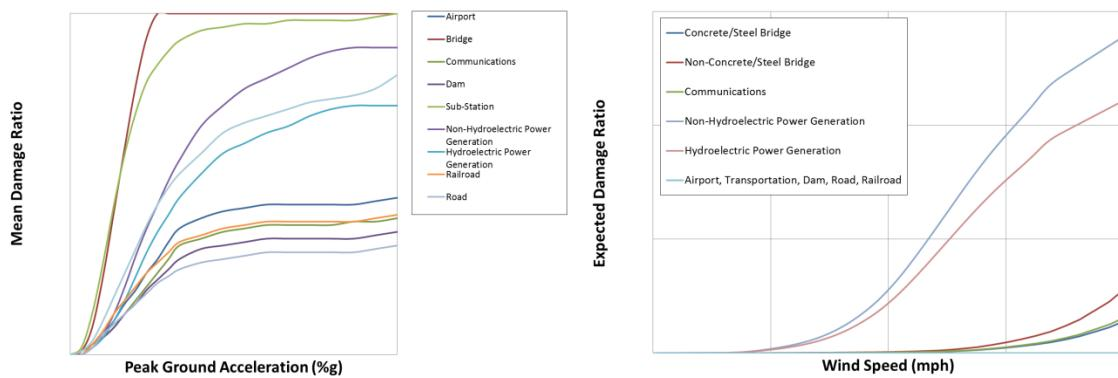
**Figure A.5. Examples of Infrastructure Damage Functions for Ground Shaking (left) and Wind Speed (right)**
