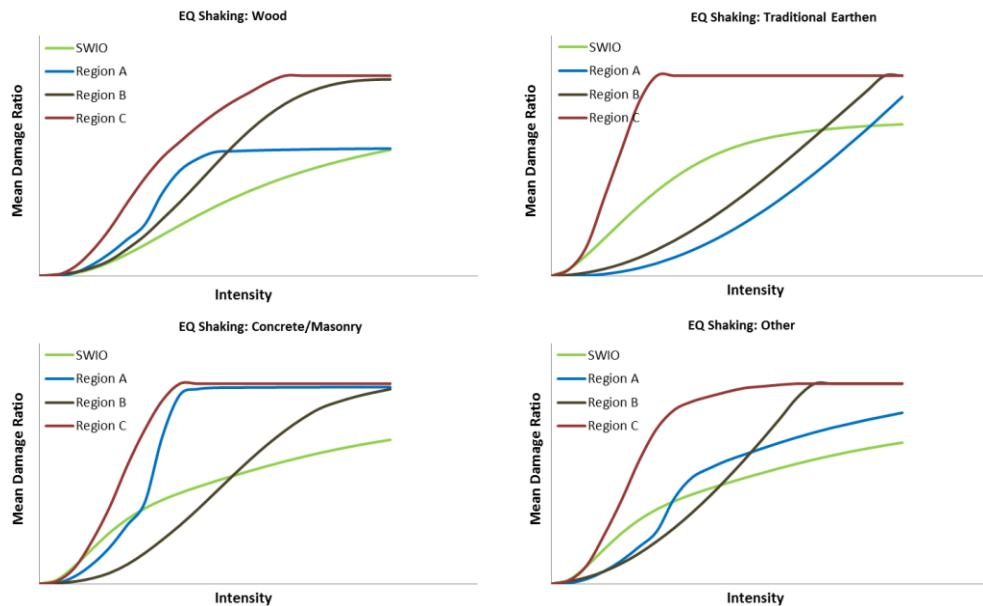
**Figure A.4. Validation of the earthquake shaking damage functions for SWIO with respect to other similar regions for timber, traditional, concrete/masonry and other construction types.**
