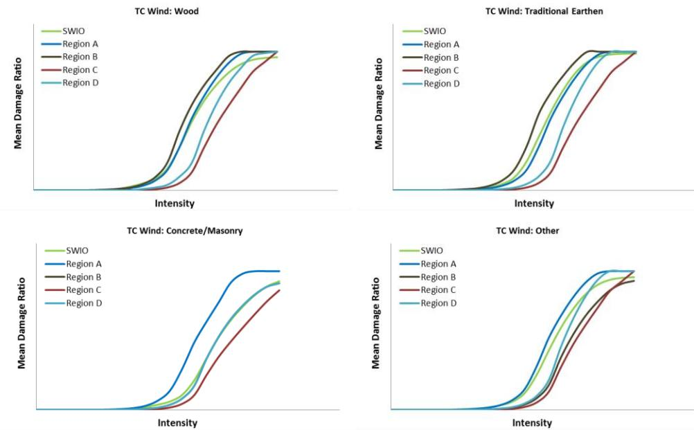
**Figure A.3. Validation of the tropical-cyclone wind damage functions for SWIO with respect to other similar regions for timber, traditional, concrete/masonry and other construction types.**
