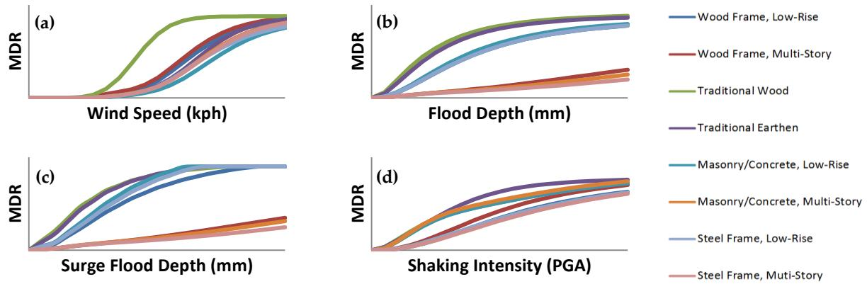
**Figure 2: Illustrative SWIO vulnerability functions for (a) tropical cyclone wind, (b) tropical cyclone precipitation flooding, (c) tropical cyclone storm surge flooding, and (d) earthquake ground shaking<sup>6</sup>**
