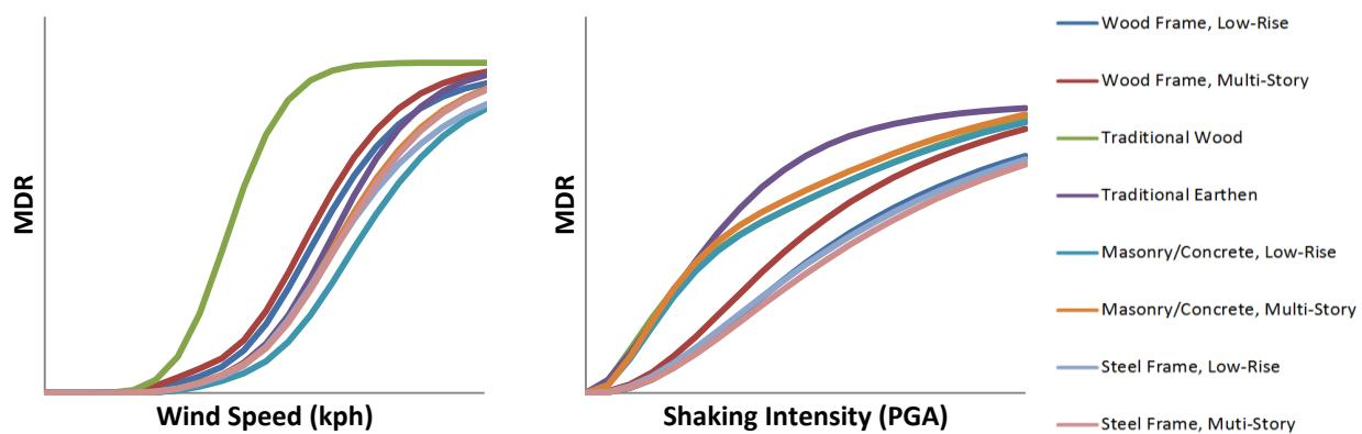
**Figure A.1. Examples of Building Damage Functions for Wind (left) and Earthquake Shaking (right)**
