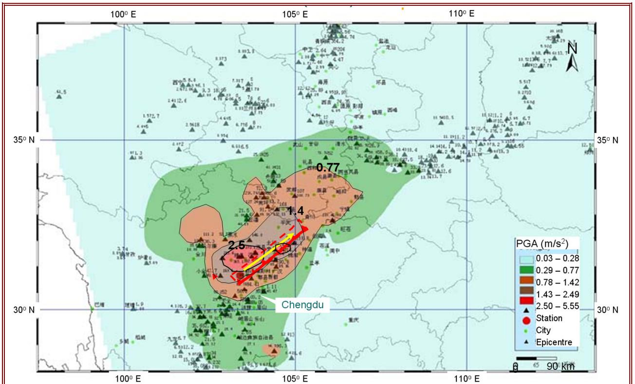
**Figure 2.3** Distribution of peak vertical ground motion (China Earthquake Data Centre, 2008).
