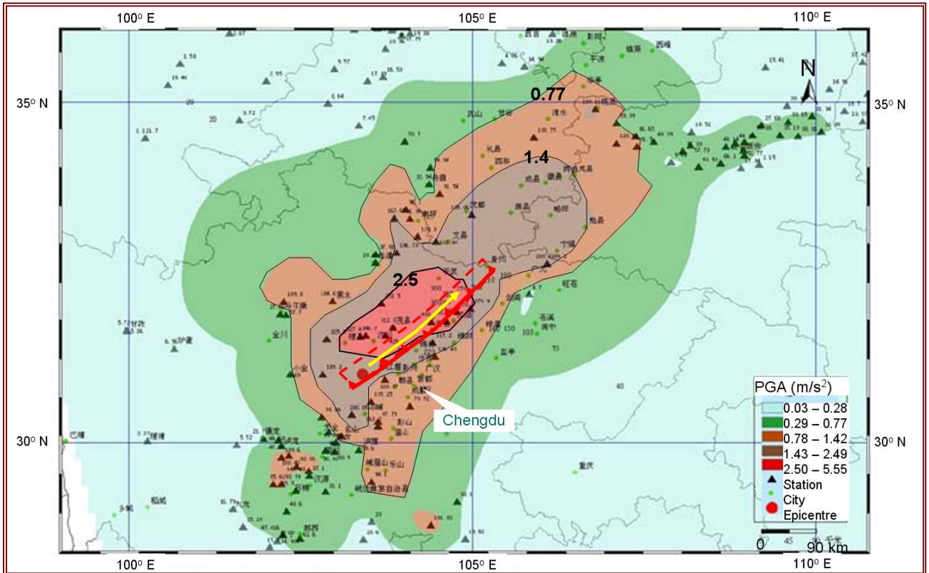
**Figure 2.2** Distribution of peak horizontal ground motion - east-west component (China Earthquake Data Centre, 2008). Red rectangle indicates surface project of fault. Dip is to northwest. Yellow arrow indicates direction of rupture.
