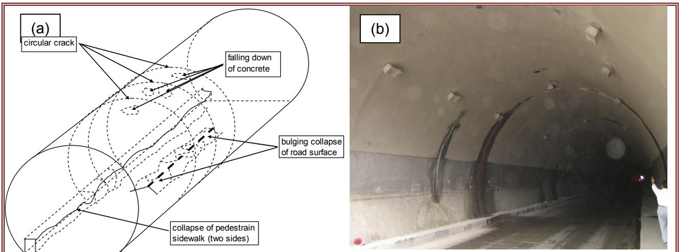
**Figure 5.3 Damage to Friendship Tunnel (Youyi Tunnel) (a) Location and types of damage including bulging of the invert, spalling from the roof, longitudinal cracks at the axis and knee and cracks and b) circumferential cracks in sprayed concrete lining.**
