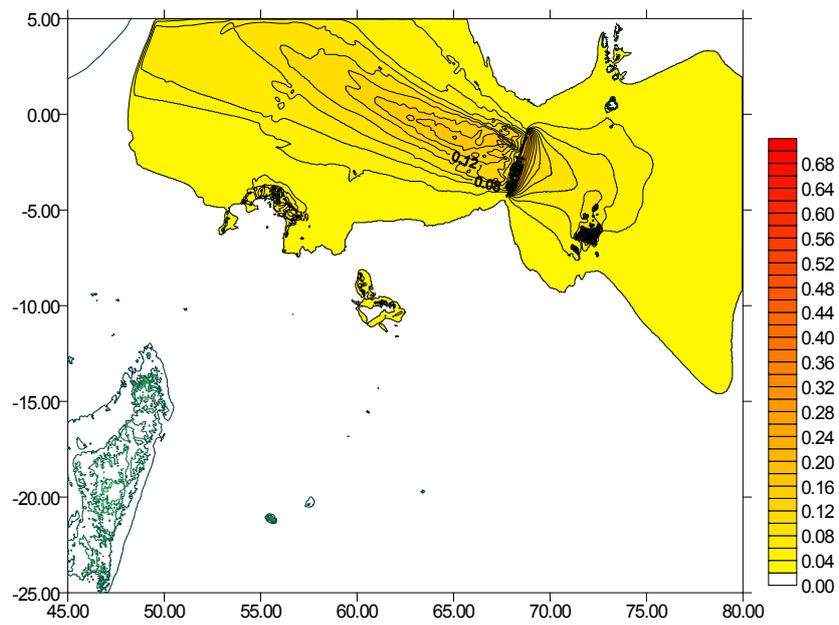
Figure 19: Simulation of the open ocean maximum wave amplitude for earthquake at 10 km with angle of dip of 70°, strike slip of 35° W and a slip of 0.5 m. The rapture zone extends from -3.2° S to -4.2°S. Model run of Avi-Nami (IOC-UNESCO, 2006)
