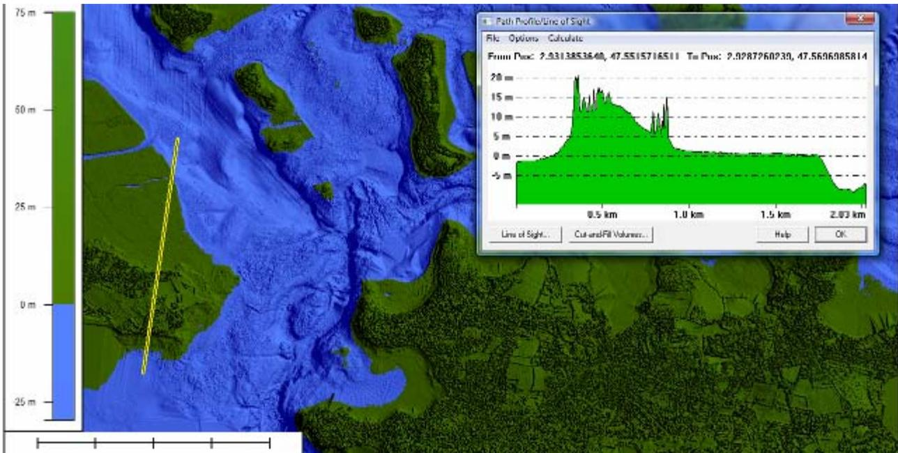
**Figure 77 : coupled topography and bathymetry of a sector in the Morbihan gulf (France). Ground resolution is 1 m.**
