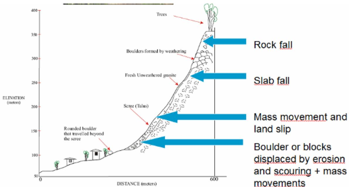
Figure 49 : typical cross section of slope showing weathered boulders on top of slope and concentration of house at the toe (modified from SEYPEC 2005).
