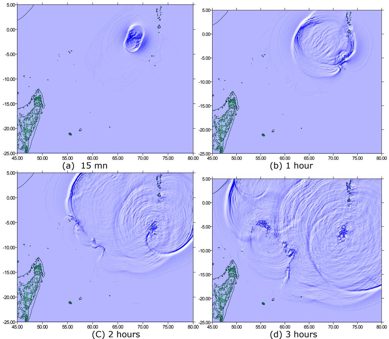
Figure 20: Tsunami propagation for Carlsberg worst case scenario at (a) 15 minutes (b) 1 hour (c) 2.0 hours and (d) 3.0 using Avi-Nami model (IOC-UNESCO, 2006)
