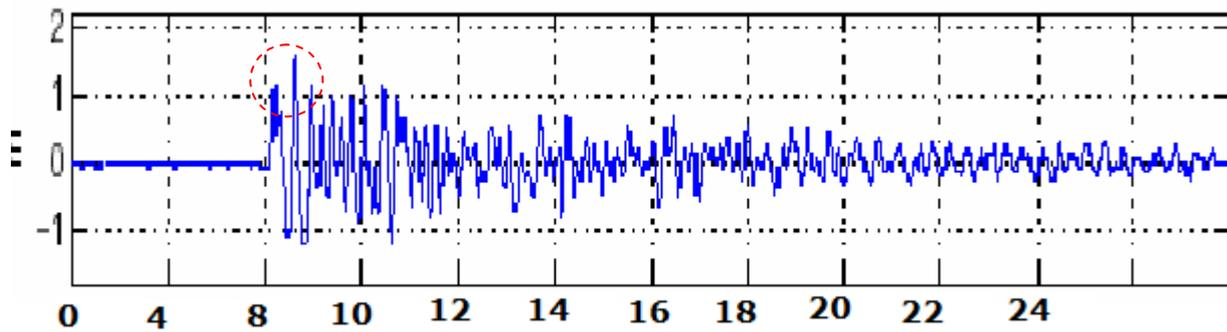
Figure 5 : Tsunami signal at Point La Rue, Mahe Seychelles with tidal oscillations removed.
