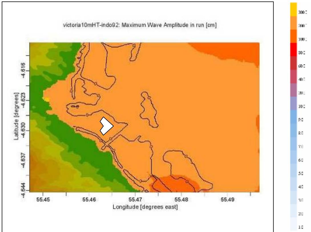
Figure 75 : maximum wave amplitude on the Victoria port for a Boxing day like tsunami arriving at high tide on the Seychelles. White polygon indicates SEYPEC tank farm. The SEYPEC site is in the range of water altitude from 2 to 3 m above high tide level.
