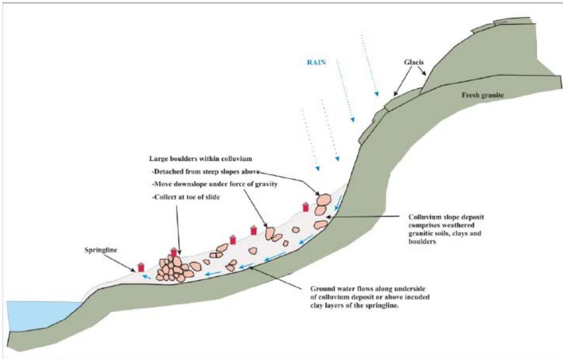
Figure 51 : diagram showing the accumulation of mixed boulders and colluviums at the base of steep granitic slope and accumulation of boulders at the toe of the slope, frequently observed on rocky shores (from Vista Do Mar SEYPEC report).
