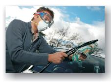
the windscreen. In heavier ashfall, driving should only be undertaken in an emergency. Use water bottles and a cloth to clean the windscreen as required. This may be every few tens of metres.
