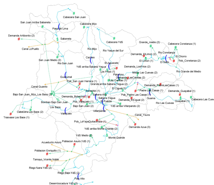
Figure 12. Schematic representation of the WEAP model for Yaque del Sur (Flores-Lopez, 2012)
